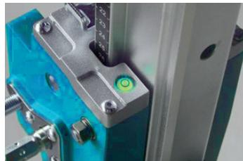
5.1.4 Using the bubble level on the carriage, adjust the four leveling bolts to achieve a good level positioning, then fully tighten the locknuts on leveling bolts. The entire stand must be mounted solidly. Both vertical and horizontal drilling share the same way to adjust a fixed drill stand.
