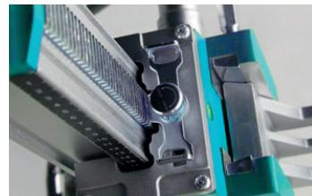
5.1.12 Quick-release bit remove tool is optional for easy removal of the drill bit.
