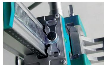
5.1.9 When mounting a 4-bolt rig-mounted type motor, to drill stand SEASTAND 250 first use 4 bolts to mount the mounting spacer to the motor. There is a  $10\times 10\times 100\text{mm}$  key on the mounting plate which can transmit the torque of the motor. Then put the mounting plate with dovetail into the cradle. Tighten the cradle lock bolt until the plate is secured in cradle.
