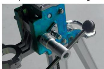
5.1.6 Check if the guidance is loose on the column. If loose, you need to adjust the 4 eccentric tensioners inside of the carriage. To adjust, use
